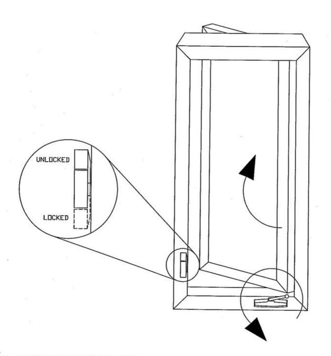
TO OPEN WINDOW, PLACE THE LOCK IN THE UNLOCKED POSITION AND TURN THE CRANK HANDLE COUNTER CLOCKWISE UNTIL WINDOW SASH REACHES A 90 DEGREE ANGLE WITH THE FRAME.
